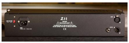
— The Weight Tank can run on US or European mains voltages — to swap, you just need to flip a switch and change a fuse in the rear-panel IEC housing.
